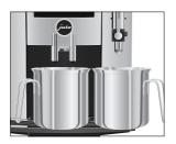
Cleaning the milk system clean it **daily** when you have been preparing milk. CAUTION If the wrong cleaning agent is used, the machine could be damaged and/or traces could be left behind in the water. Use only original JURA maintenance products. **j** JURA milk system cleaner is available from specialised dealers. **i** To clean the milk system, use the container supplied.
